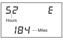
of miles (or kilometers) that the walking belt has moved. An "E" for English miles or an "M" for metric kilometers will appear in the Pace/Speed zone. Press the Speed increase button to change the unit of measurement if desired.
